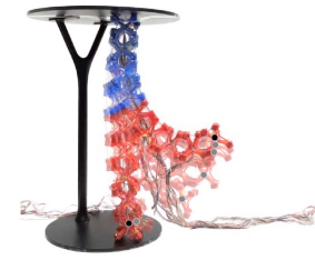
Fig. 7. Maximum reach of the arm in the x direction; black dots show a point on the center of the end effector).
